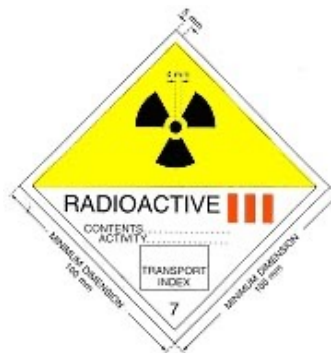
FIGURE 4: Category III-YELLOW label. The background color of the upper half of the label shall be yellow and of the lower half white, the color of the trefoil and the printing shall be black, and the color of the category bars shall be red.
