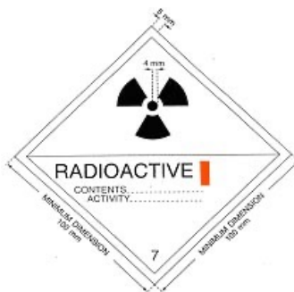
FIGURE 2: Category I-WHITE label. The background color of the label shall be white, the color of the trefoil and the printing shall be black, and the color of the category bar shall be red.
