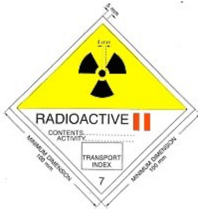
FIGURE 3: Category II-YELLOW label. The background color of the upper half of the label shall be yellow and of the lower half white, the color of the trefoil and the printing shall be black, and the color of the category bars shall be red.
