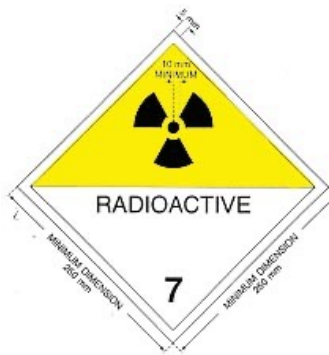
FIGURE 6: Placard. Minimum dimensions are given; when larger dimension is used the relative proportions must be maintained. The figure “7” shall not be less than 25 mm high. The background color of the upper half of the placard shall be yellow and of the lower half white, the color of the trefoil and the printing shall be black. The use of the word “RADIOACTIVE” in the bottom half is optional to allow the alternative use of this placard to display the appropriate United Nations Number for the consignment.
